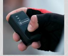
You will receive a GPS tracker from "Follow my challenge". For the GPS signal to be transmitted correctly, the tracker must have battery power (USB-A to USB-C cable) and be positioned at the top of a pannier. It is the rider's responsibility to ensure that he or she has sufficient battery power.
